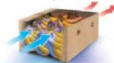
5 The SmartAir System forces pressurized air through every square inch of the load, precisely controlling product temperature and respiration, then returning air to the mixing chamber.
